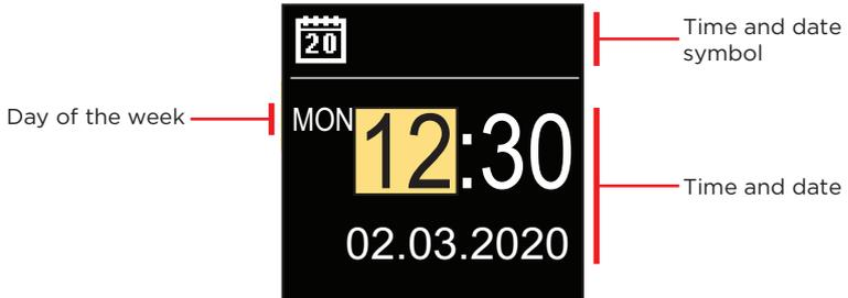
With the buttons  $\ominus$  and  $\oplus$  you can change the value and with the button  $\odot$  you can move on to the next data. Exit the screen with the button  $\odot$ .
