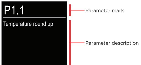
With the  $\ominus$  and  $\oplus$  buttons navigate through the parameters in the selected group. The parameter you want to change is selected by pressing the  $\odot$  button. The parameter setting screen, which can take the form of a menu or a slider, opens.
