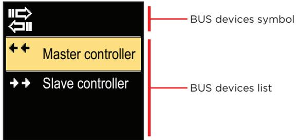
Navigate through the list with the  $\ominus$  and  $\oplus$  buttons. Exit the screen with the button  $\odot$ .
