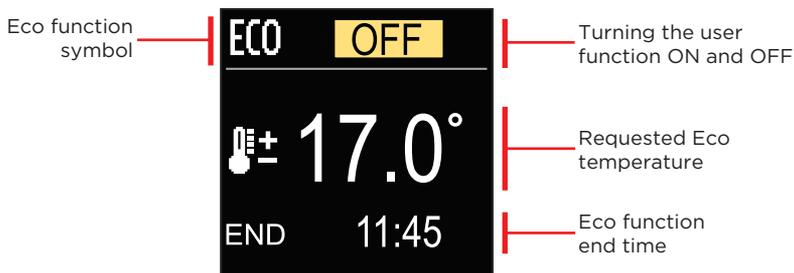
With the buttons ⊖ and ⊕ you can change the setting value and with the button ⦿ you can move on to the next setting.
