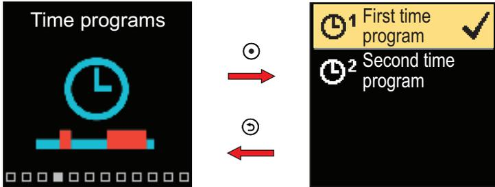
Navigate through the menu with the  $\ominus$  and  $\oplus$  buttons. With the button  $\odot$  you can select the time program for operation and with the button  $\odot$  you can enter the setting of the selected time program.
