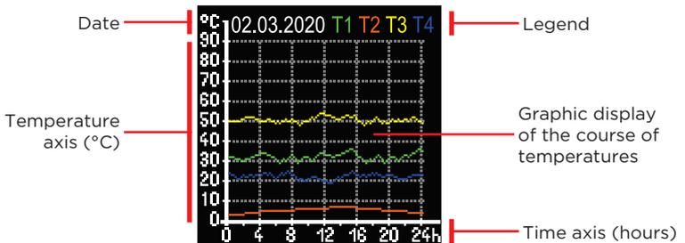
With the buttons  $\ominus$  and  $\oplus$  you can browse the temperature graphs for the last 7 days of operation. Exit the setting by pressing  $\odot$ .
