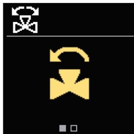
You can select the opening direction of the mixing valve. Use the buttons  $\ominus$  and  $\oplus$  to navigate between directions.
