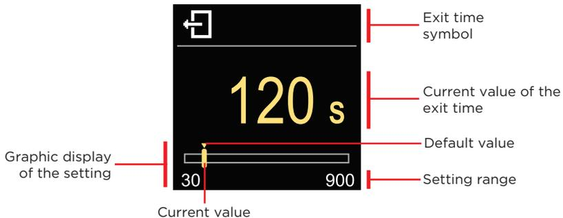
With the  $\ominus$  and  $\oplus$  buttons you can set the automatic exit time and confirm it with the  $\odot$  button. Exit the setting with the  $\odot$  button.
