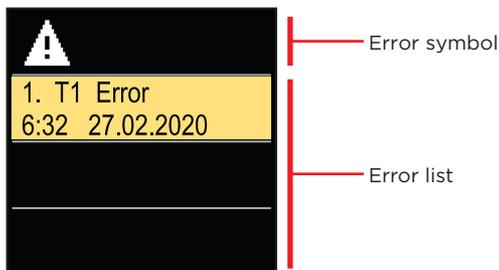
Navigate through the error list with the  $\ominus$  and  $\oplus$  buttons. Exit the screen with the button  $\odot$ .
