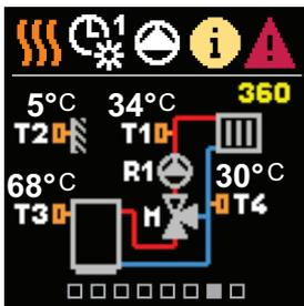
Hydraulic scheme with screen showing the measured temperatures
