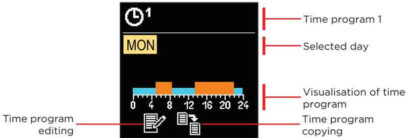
With the buttons  $\ominus$  and  $\oplus$  you can select the day for which you want to edit or copy the time program and confirm it with the button  $\odot$ . Now, with the buttons  $\ominus$  and  $\oplus$  select the icon to edit or copy the time program and confirm it with the button  $\odot$ .
