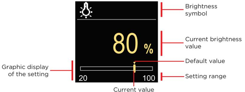
Use the  $\ominus$  and  $\oplus$  buttons to adjust the brightness and confirm it with the  $\odot$  button. Exit the setting with the  $\odot$  button.
