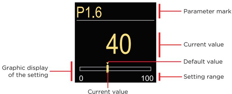
Use the  $\ominus$  and  $\oplus$  buttons to set the requested value and confirm it with the  $\odot$  button. Exit the setting with the  $\odot$  button.
