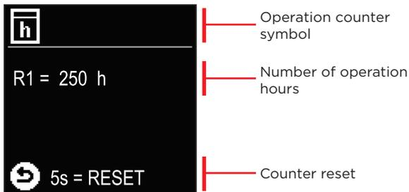
By pressing the button
