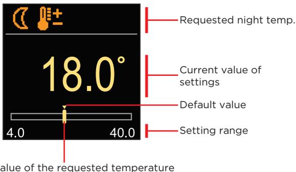
Use the  $\ominus$  and  $\oplus$  buttons to select the requested temperature and confirm it with the  $\odot$  button. Exit the setting with the  $\odot$  button.
