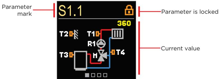
With the  $\ominus$  and  $\oplus$  buttons navigate through the parameters in the selected group. The parameter you want to change is selected by pressing the  $\odot$  button.
