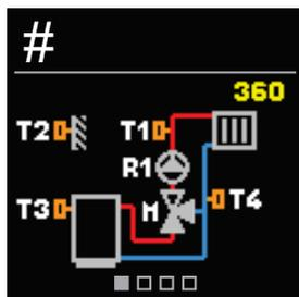
You can select the hydraulic scheme for the controller operation. Use the buttons  $\ominus$  and  $\oplus$  to navigate between schemes.
