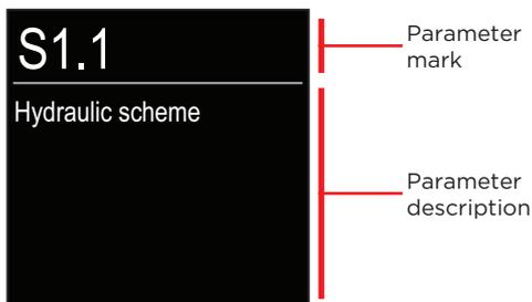
With the  $\ominus$  and  $\oplus$  buttons navigate through the parameters in the selected group. The parameter you want to change is selected by pressing the  $\odot$  button. The parameter setting screen opens.
