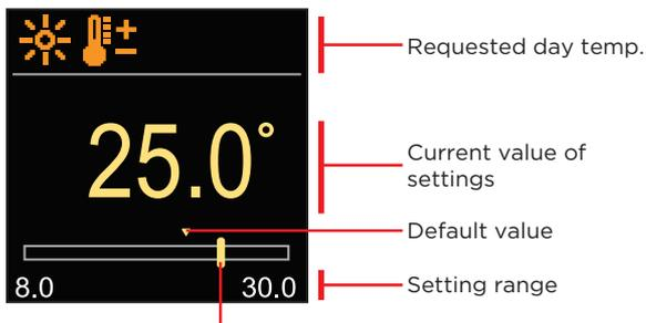
Use the  $\ominus$  and  $\oplus$  buttons to select the requested temperature and confirm it with the  $\odot$  button. Exit the setting with the  $\odot$  button.
