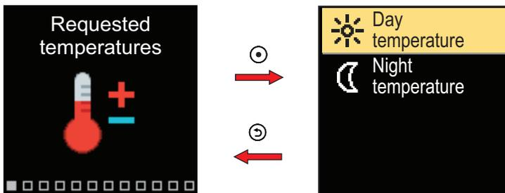
Navigate through the menu with the  $\ominus$  and  $\oplus$  buttons and use the  $\odot$  button to confirm your selection. A new screen with temperatures will open.
