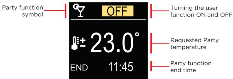
With the buttons  $\ominus$  and  $\oplus$  you can change the setting value and with the button  $\odot$  you can move on to the next setting.
