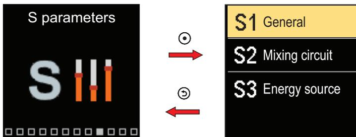
Navigate through the menu with the  $\ominus$  and  $\oplus$  buttons. When you use the  $\odot$  button to select the requested parameter group, a display will open describing the first parameter in the group.
