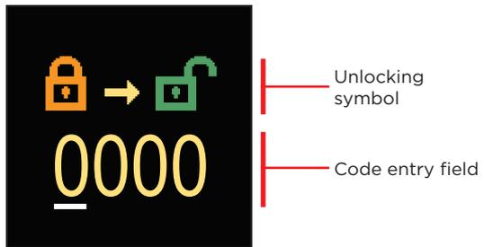
With the buttons  $\ominus$  and  $\oplus$  you can change the value and with the button  $\odot$  you can move on to the next position and confirm the unlocking. Exit the screen with the button  $\odot$ .
