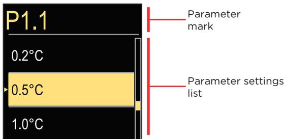
Use the  $\ominus$  and  $\oplus$  buttons to select the requested setting and confirm it with the  $\odot$  button. Exit the setting with the  $\odot$  button.
