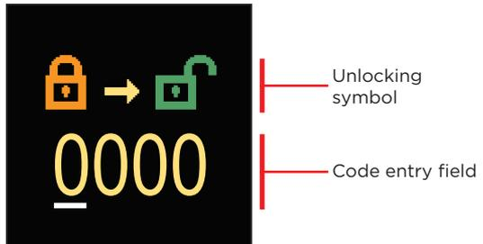
With the buttons  $\ominus$  and  $\oplus$  you change the value and with the button  $\odot$  you move on to the next position and confirm the unlocking.
