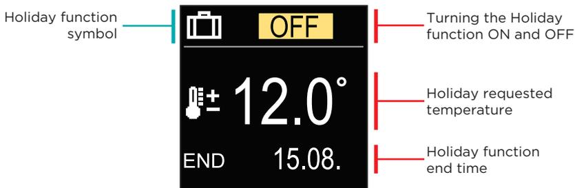
With the buttons ⊖ and ⊕ you can change the setting value and with the button ⦿ you can move on to the next setting.
