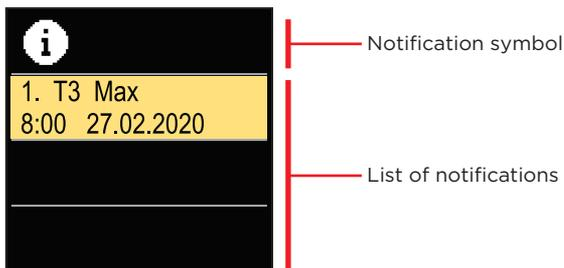
Navigate through the notifications with the  $\ominus$  and  $\oplus$  buttons. Exit the screen with the button  $\odot$ .
