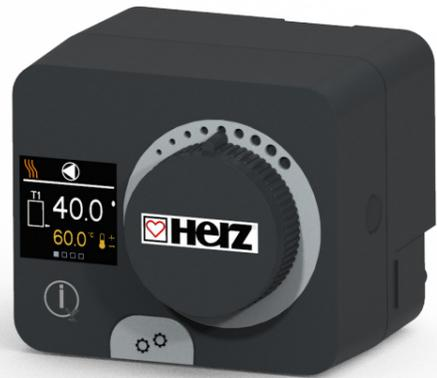
The smartcontrol plus is a compact weather-controlled heating controller built into the motor drive housing. It allows direct mounting on more than 20 mixing valves from different manufacturers. The controller can also be used in systems without an external sensor, but in this case the use of a room unit is mandatory.
