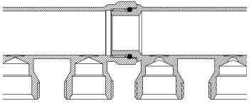
Manifolds with isolation 20° inclined valves
