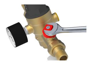
The handle is clearly marked to indicate the valve's status: when the marking is perpendicular to the flow or pipe, the valve is closed; when aligned parallel, the valve is open. These markings provide a clear visual reference, aiding in the correct operation and maintenance of the heating system.
