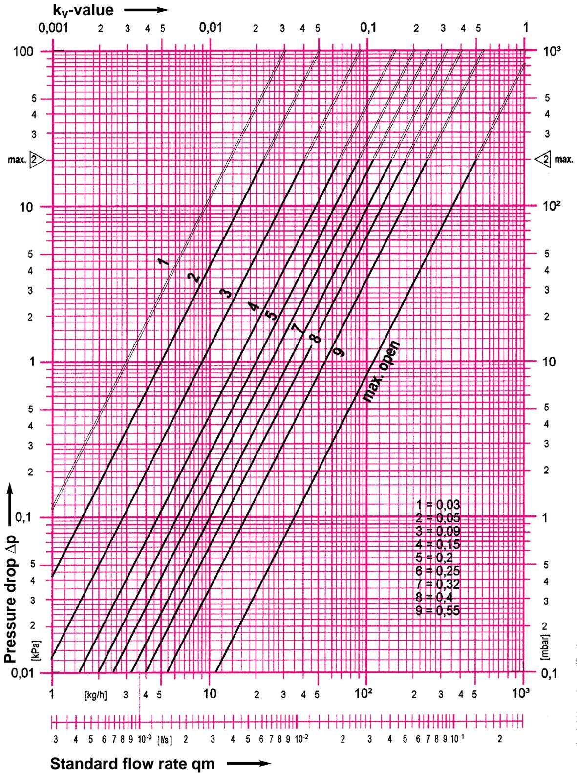
The characteristics "1–9" are valid for nominal lift (2 K) of the valve cone.
