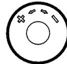
In the exceptional case that the HERZ thermostatic valve lower part is not equipped with a HERZ thermostatic head, the HERZ-TS handwheel is used to replace the screw cap.
